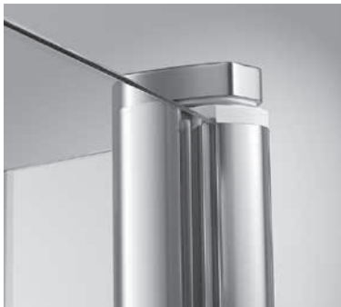
The RAISE-LOWER hinge provides simple opening and closing of the doors. When opening, the swinging door is raised gently. When closed, the door is lowered again.
